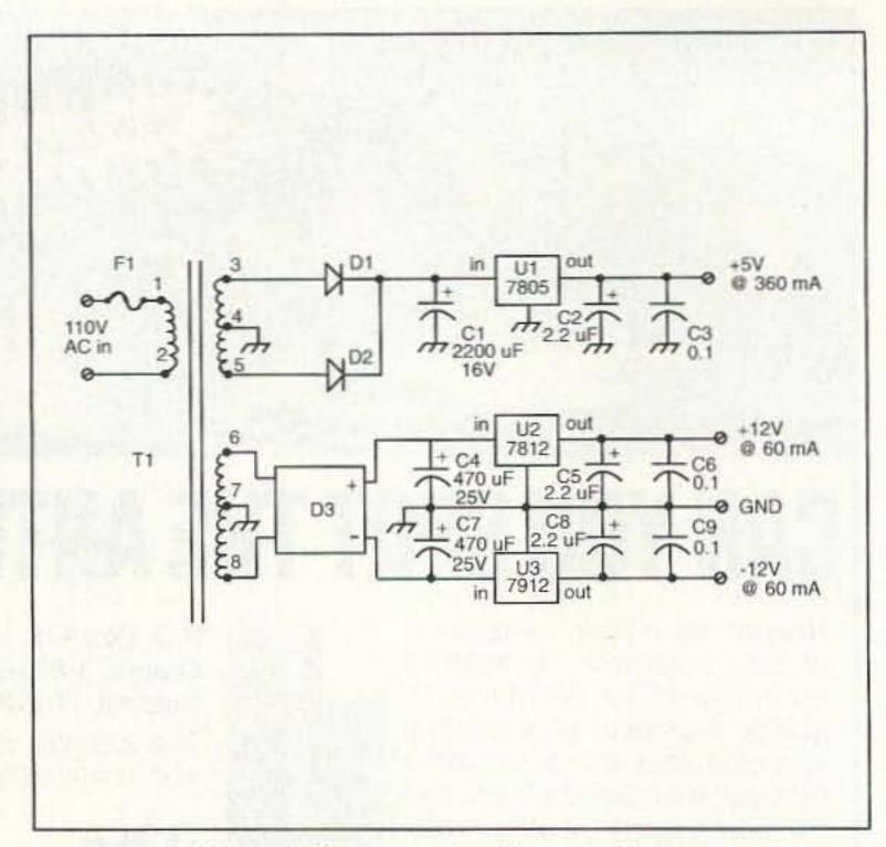
Figure 4. Power supply schematic diagram.
